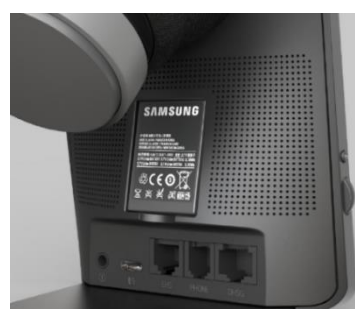
Fig. 13 Spare battery charging.
