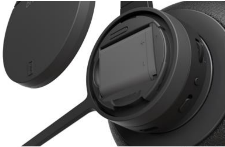
Fig. 10 Battery lid removed.
